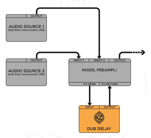
In this way, all the sources are mixed and managed directly by the mixing tool. It is the mixing equipment that sends more or less of each source into the input of the effect by its "Effect Send" output. It is then necessary to have a mixing desk have this feature to use it in such setup.
