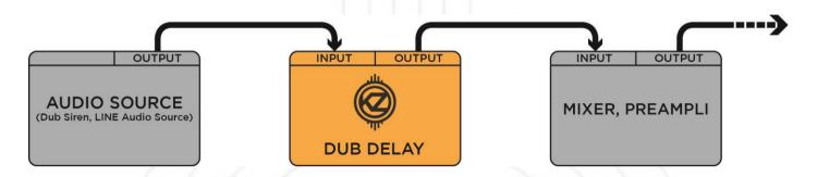
This setup is the simplest, but does not allow using the effect on multiple sources in the same time.
