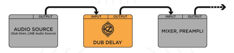
This setup is the simplest, but does not allow using the effect on multiple sources in the same time.
